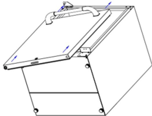
Slide the door up onto the top left pivot hinge and allow door to lay flat.
