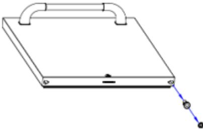
Remove the spring tension plug (off white plastic) and bearing from the bottom right of door.
