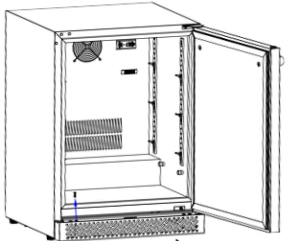
Remove and retain the screw holding the top of the Kickplate.
