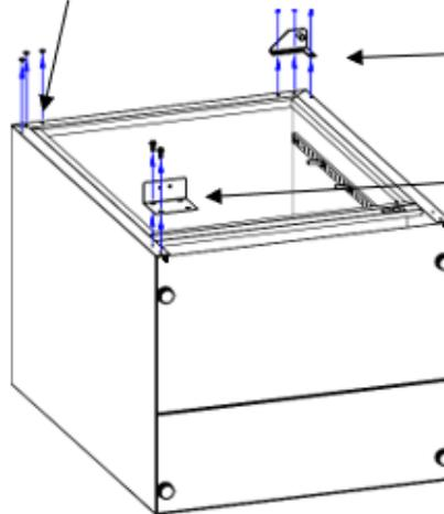
Remove top right pivot hinge (x3 screws)
