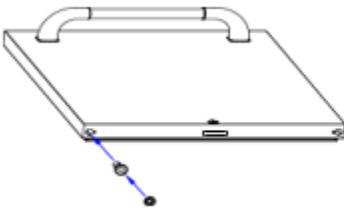
Install the black spring tension plug (supplied in parts bag) to the bottom left of the door.
