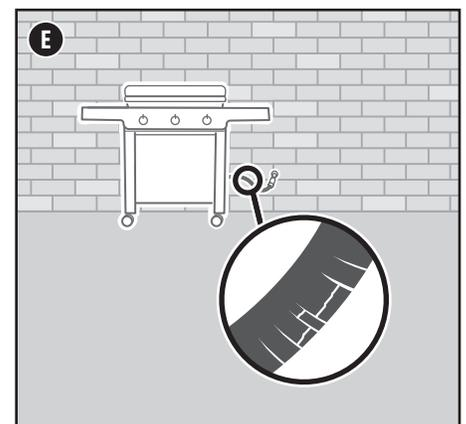
**⚠ DANGER:** Do not use a flame to check for gas leaks. Be sure there are no sparks or open flames in the area while you check for leaks.
