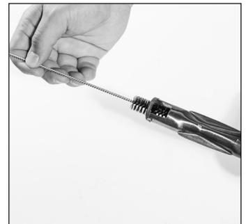
**STEP 04** Brush entire outer surface of burner to remove grime.
