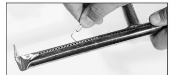
**STEP 06** Carefully replace burners and reattach, with attention to the location of the ignition needle.
