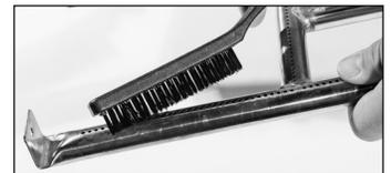
**STEP 05** Clean any blocked ports with stiff wire such as an open paper clip.
