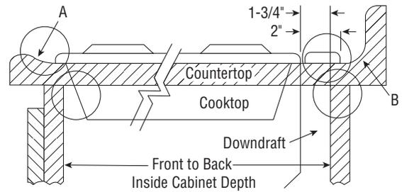
Refer to the cooktop installation instructions for dimensions of cooktop, countertop cut-out, and cabinet requirements. The 2730 and 2736 can be installed in most standard 30" and 36" wide cabinets.
