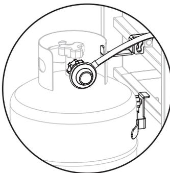
The safety relief valve must face away from the user while the appliance is in use.
