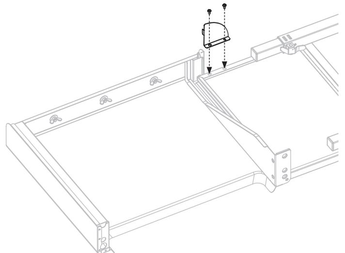
**STEP 14** Screw two (2) M6 step bolts [f.] into the top holes of the right side shelf.
