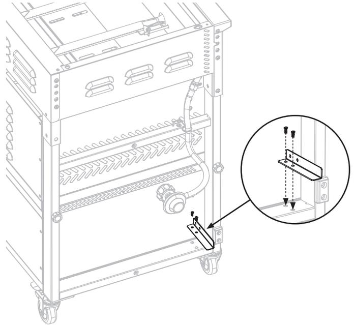
**STEP 04** Use two (2) M6x12 bolts [a.] to attach one (1) holding bracket to the right cart panel.
