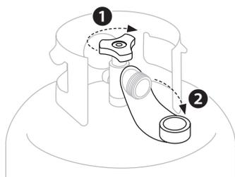
**STEP 02** Hold the regulator in a straight line with the Type 1 valve outlet so as not to cross thread the connection.
