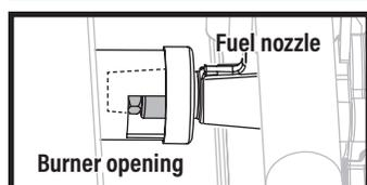
**⚠** Ensure that the gas rail fuel nozzle orifice is correctly engaged within the burner opening.
