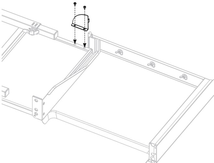
**STEP 13** Use two (2) M5x15 bolts [c.] to attach the left rotation bracket to the left table.
