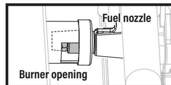
⚠ The gas rail fuel nozzle must be reengaged within the burner opening.
