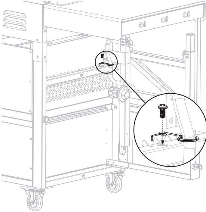
**STEP 19** Use one (1) M6x12 bolt [a.] to attach the LPG hook to the left leg assembly.
