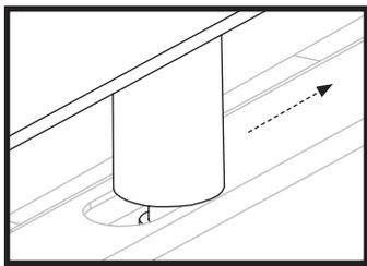
**STEP 23** Hang the grease cup with grease cup liner in the slot at the back of the griddle body.
