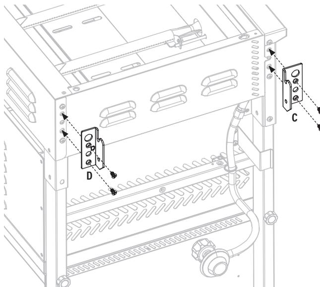
**STEP 08** Use three (3) wing nuts [e.], three washers [h.], three slotted washers [i.], and three (3) side shelf pegs [b.] to the right side shelf.
