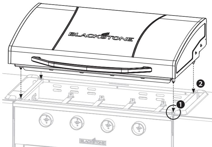
❶ Place the two front pins into the front locking holes and push the griddle top back.
