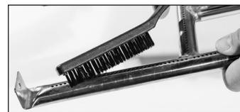
**STEP 05** Clean any blocked ports with stiff wire such as an open paper clip.
