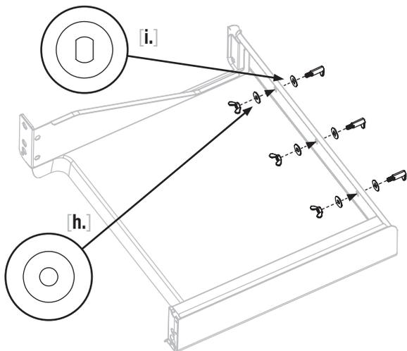
**STEP 09** Use three (3) wing nuts [e.], three washers [h.], three slotted washers [i.], and three (3) side shelf pegs [b.] to the left side shelf.
