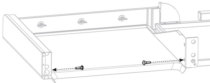
**STEP 16** Hook the right side shelf's upper step bolts on the side shelf brackets. Use two (2) M6 step bolts [f.] to secure the side shelf to the side shelf brackets.
