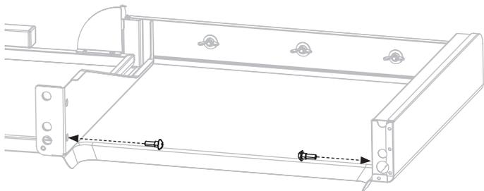
**STEP 15** Screw two (2) M6 step bolts [f.] into the top holes of the left side shelf.
