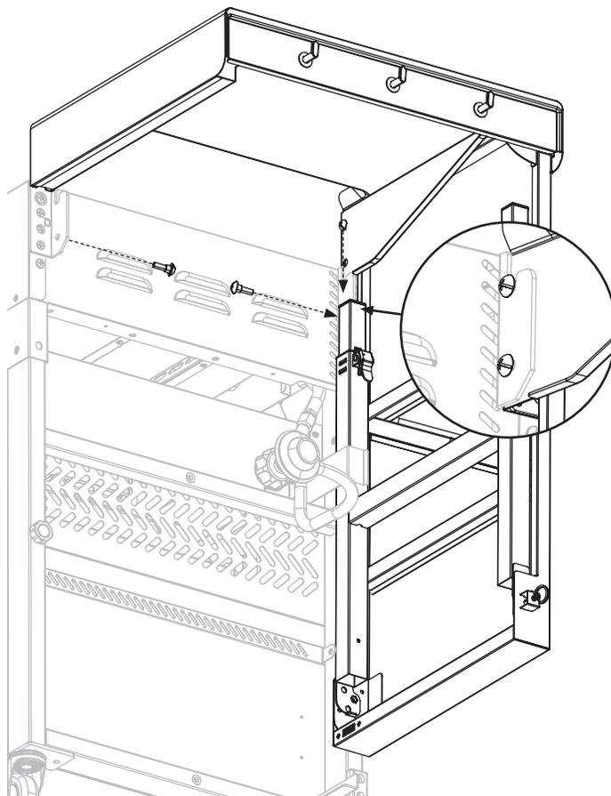
**STEP 18** Use one (1) M6x12 bolt [a.] to attach the regulator hose retaining wire to the left leg assembly.
