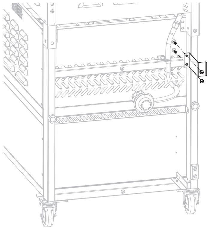
**STEP 06** Use four (4) M6x12 countersunk bolts [g.] to attach side shelf brackets (A) and (B) to the right side of the griddle body.
