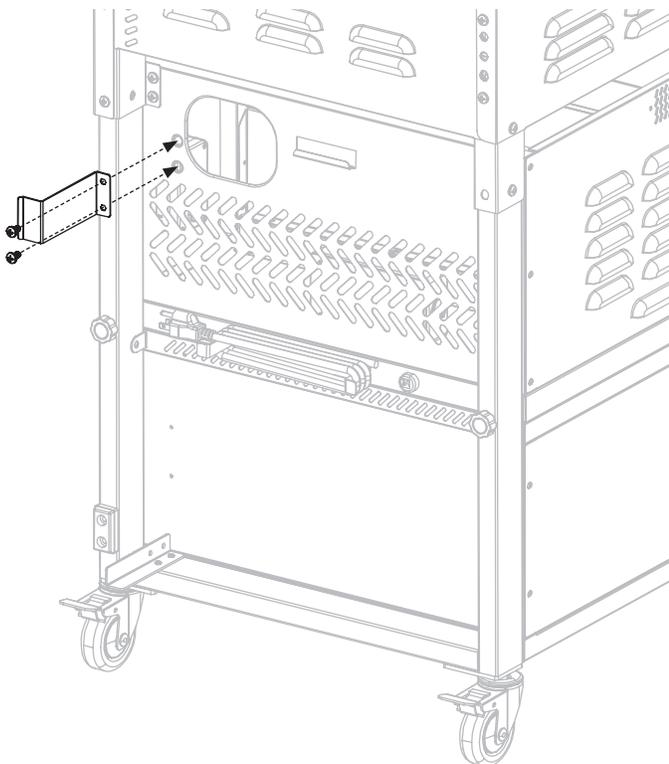
**STEP 05** Use two (2) M6x12 bolts [a.] to attach one (1) holding bracket to the left cart panel.
