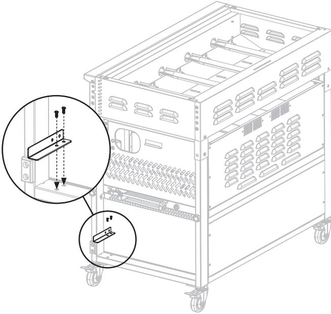
**STEP 03** Use two (2) M5x15 bolts [c.] to attach one (1) stopper plate to the left leg assembly.
