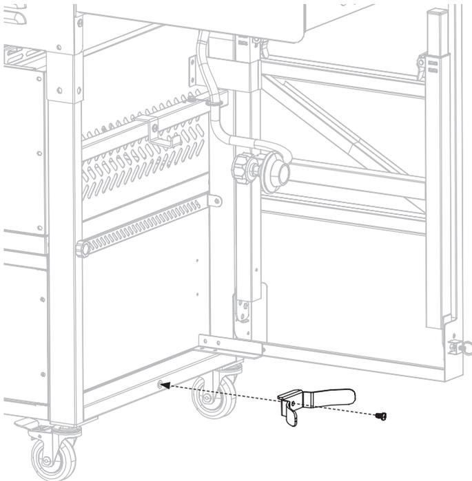
**STEP 21** Use four (4) M6x12 bolts [a.] to attach the two (2) mica sheets and the hood handle to the front of the hood.
