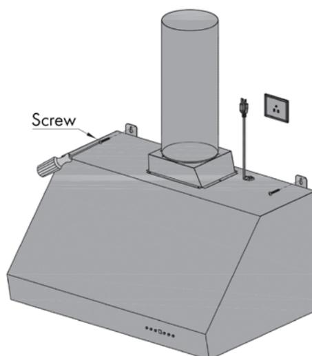
9. Use a second person to hold the hood in place while you align the hood-mounting brackets to the partially fastened screws on the wall.
