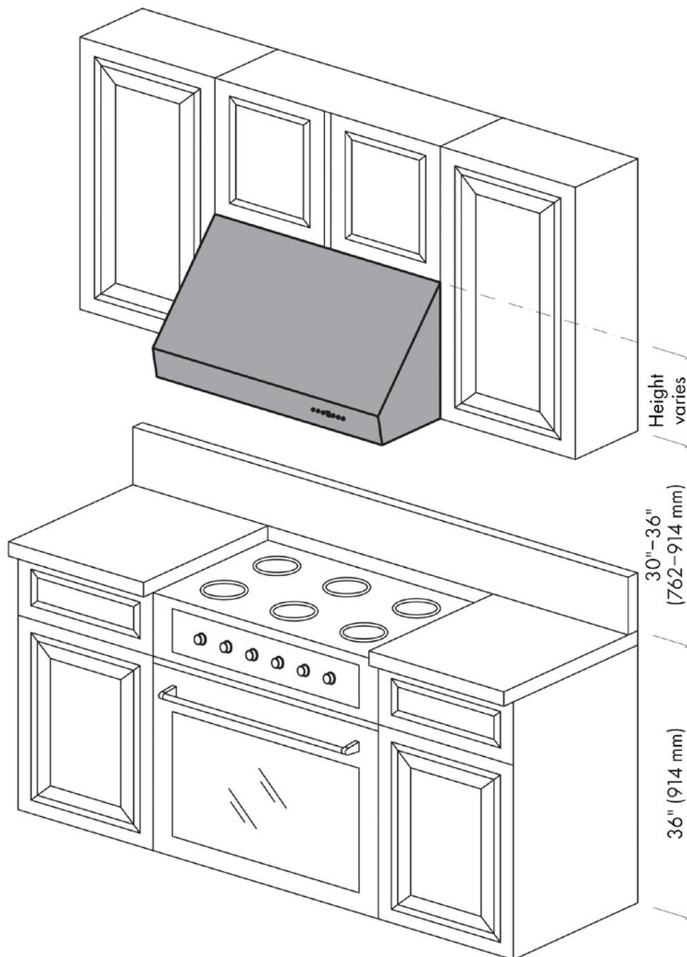
**NOTE:** The recommended height to install your hood is 30" (762 mm) minimum and 36" (914 mm) maximum above your range top or cook top. For outdoor installation, the hood should be installed between 36" (914 mm) and 42" (1067 mm) above the grill. These distances allow for optimal venting efficiency. Consult an HVAC or installation professional for ventilation advice.
