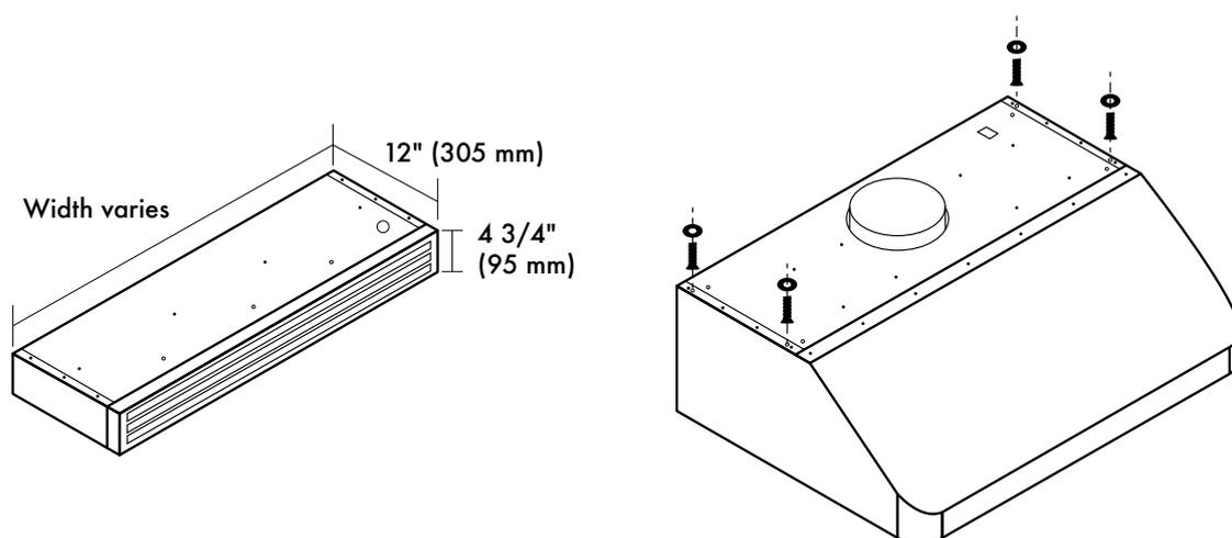
3. Secure the recirculating kit to the range hood with the provided screws and washers as shown below. Once secure, fully tightening each screw until the recirculating kit is flush with the range hood. Use care to not overtighten.
