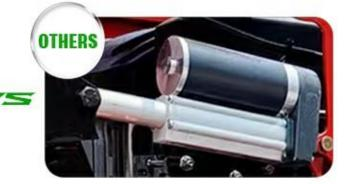
The opponent push rod motor has small power, small diameter, poor heat dissipation of the plastic shell, and poor strength of the aluminum push rod.
