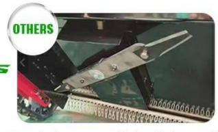
Regular lawn mower blades; blades are thin and don't spin. Ordinary screws are easy to fall off and break.
