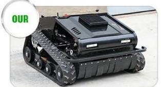
The high-strength steel pipe welding of the whole vehicle structure, double-row wheel design and crawler shock absorption system ensure stable operation on any surface. And has anti-rollover protection.
