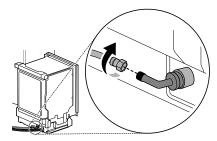
Tighten both connections using two adjustable wrenches to avoid putting stress on the water inlet valve.
