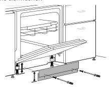
**2** Attach a custom toe kick. If needed, use a saw to cut a notch in the top of the custom toe kick to provide clearance for the cabinet panel when opening the door.
