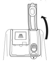
Add a liquid rinse aid to the maximum fill level. Allow the rinse aid to settle in the dispenser while filling, or air bubbles may result in poor drying performance. Avoid overfilling the dispenser.
