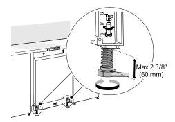
The adjustments work identically for both front leveling feet.  When a flat-blade screwdriver is unavailable, use a 1/4" square drive wrench ① or 3/8" square drive wrench ② with 1/2" socket ③ to turn the front leveling feet and adjust the front of the tub.
