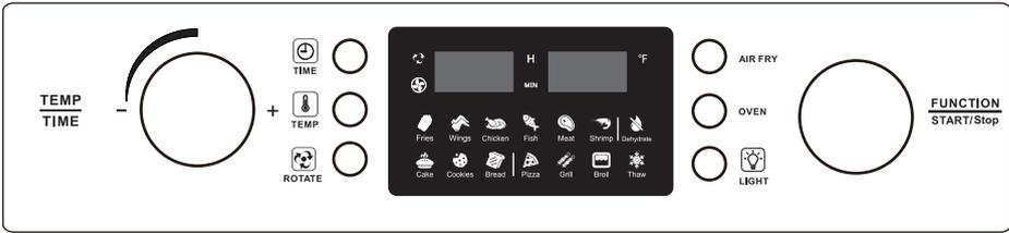
When the appliance is initially plugged in, the display will show "--" on the control panel display. When the Air Fry or Oven programs are selected, the time will show on the left side of the display and the temperature will show on the right side.
