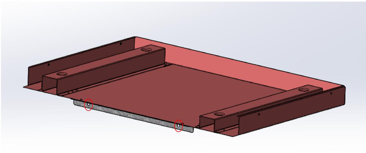
4. Install the frame with brackets to the cabinetry. Use the 4 holes (circled below in RED) to mount to the front of the cabinetry.
