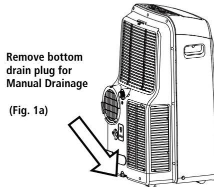
Remove bottom drain plug for Manual Drainage
