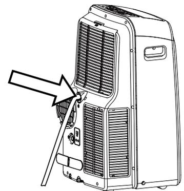
Attach drain hose for Continuous Drainage
