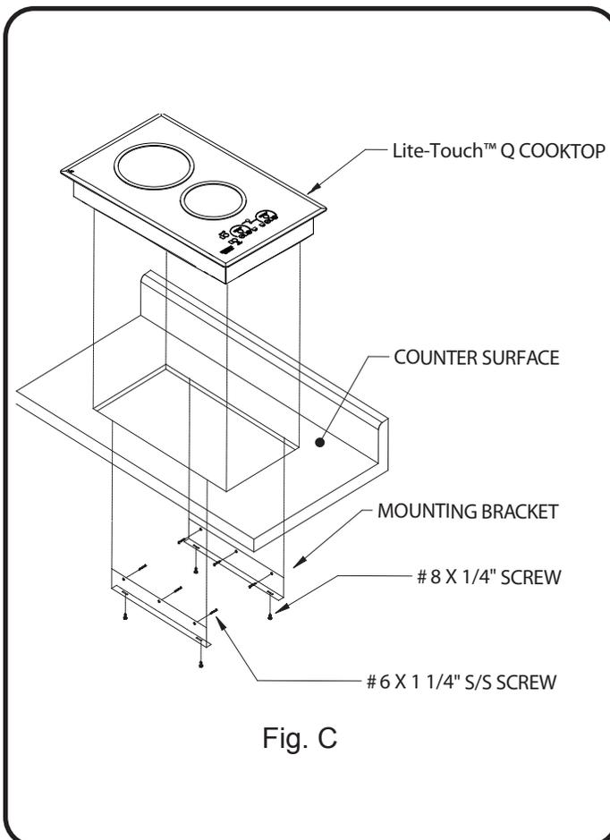
Attach the two mounting brackets as shown (see Fig. C) to the inside vertical surface of the cutout. The brackets are to be mounted on opposing sides. Center the bracket in the opening, **flush with the countertop** and secure with #6 self-tapping screws that are provided. Position the cooktop in the cutout opening and press firmly on all sides to seal the glass into the bedding compound. Secure the cooktop to the brackets from underneath with the small sheet metal screws that are supplied.
