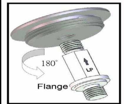
Step 3: Turn the Stem 180° so that the Flange is at The Bottom.
