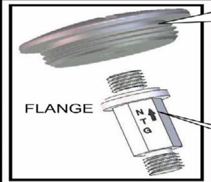
Step 2: Unscrew the Stem from the cap
