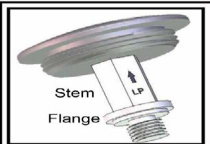
Step 4: Screw the Stem back into the Cap and then reinstall the Cap/Stem Assembly back into the Regulator.
