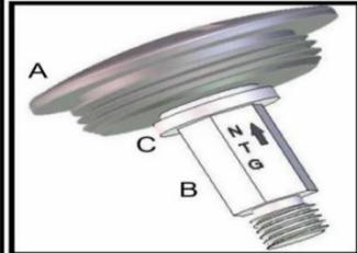
Cap is attached to regulator and in this picture it is shown as "set to Natural Gas".
