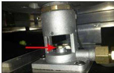
3. Remove orifice and replace with orifice of desired gas type and reassemble.
