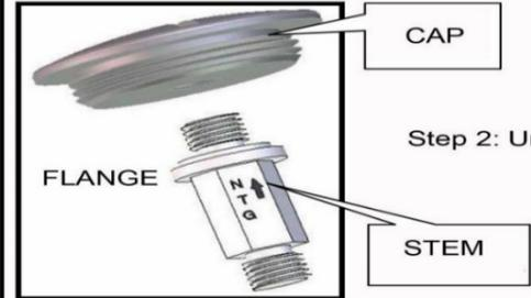
Step 2: Unscrew the Stem from the cap
