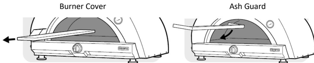
**Burner Cover** – When using wood in the oven, install the burner cover to prevent ash from getting in the burner. The burner cover is made of stone to expand the cooking area.
