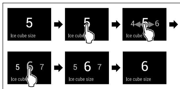
Fig. 65 Example illustration: Switching from value 5 to value 6.
