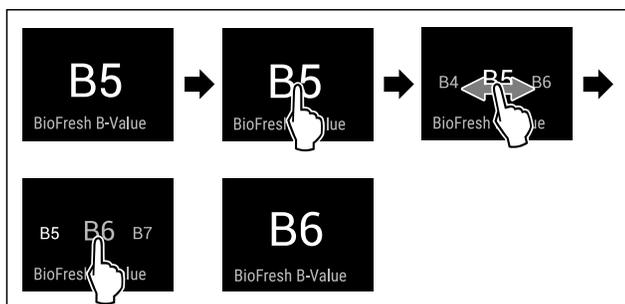
Fig. 29 Example illustration: Switching from B5 to B6.
