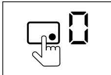
Press the button for the desired cooking zone to set the power level. Burner display '0' will blink.
