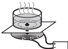
Instead of heating the ceramic glass, this method heats the base of the pan immediately, saving time and energy. Since the heat required for cooking is generated directly in the base of the pan, the cooking zone itself warms up only slightly. The cooktop does become hot when heat is transferred from the cookware.
