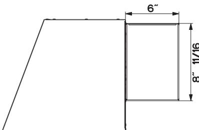
Install to the Roof or Wall attach ductwork.
