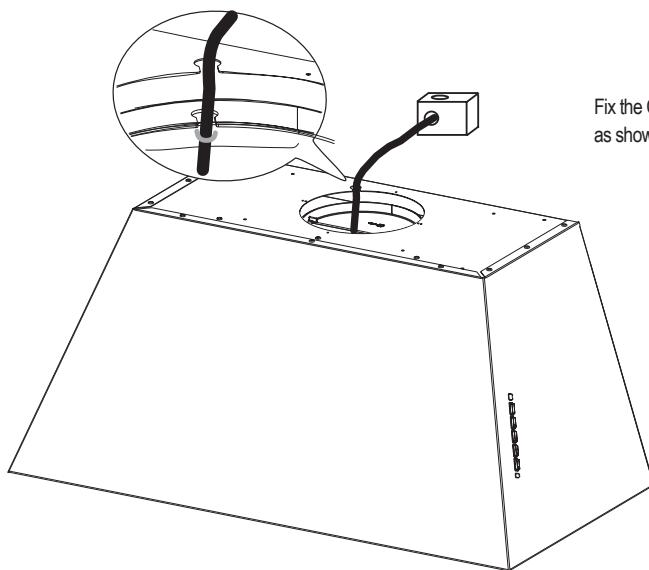
Fix the Cable in the hole on the Top of the Hood
