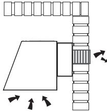
Before fixing the Body Hood to the Rear Section, Unscrew the 2 screws to fix the Blower.
