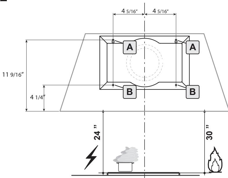
Mark the wall where indicated (A), 11 9/16" above the horizontal line and at 4 5/16" distance on the left and right of vertical line. Checking that the two marks are level.
