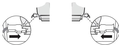
From inside the hood re-connect the Connectors on the left and right side shown in the image above.
