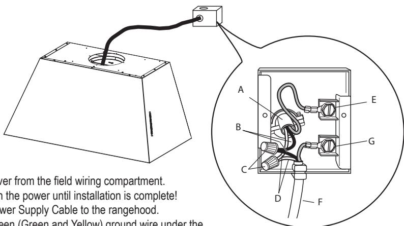
Remove the cover from the field wiring compartment.
