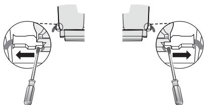
From inside the hood, use a flat head screwdriver as shown in image above, to disconnect the left and right Connectors from the blower.
