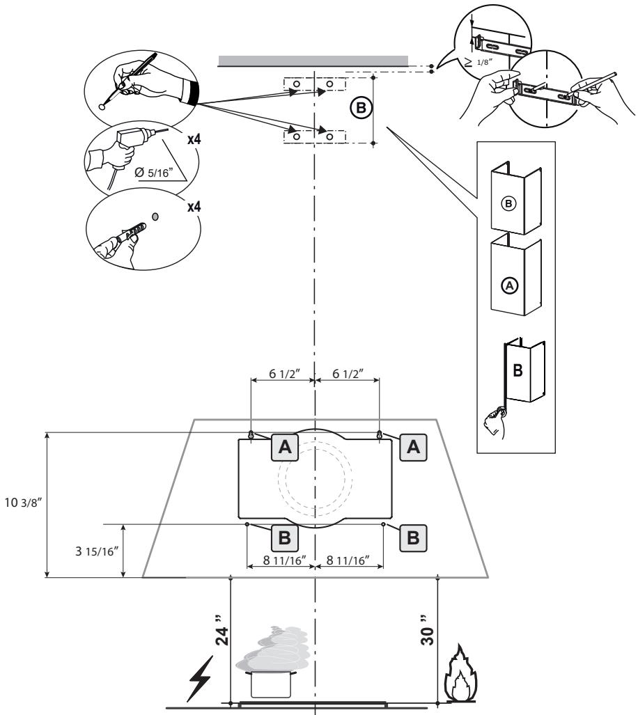
Mark the wall where indicated (A), 10 3/8" above the horizontal line and at 6 1/2" distance on the left and right of vertical line. Checking that the two marks are level.
