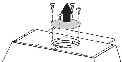
Remove the 4 screws as shown and take off the cover plates.
