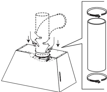
Install Roof or Wall Cap purchased separately. Connect the 6" metal ductwork to the Roof or Wall Cap and then attach ductwork.
