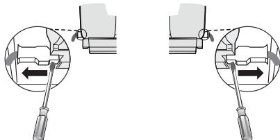
From inside the hood, use a flat head screwdriver as shown in image above, to disconnect the left and right Connectors from the blower.
