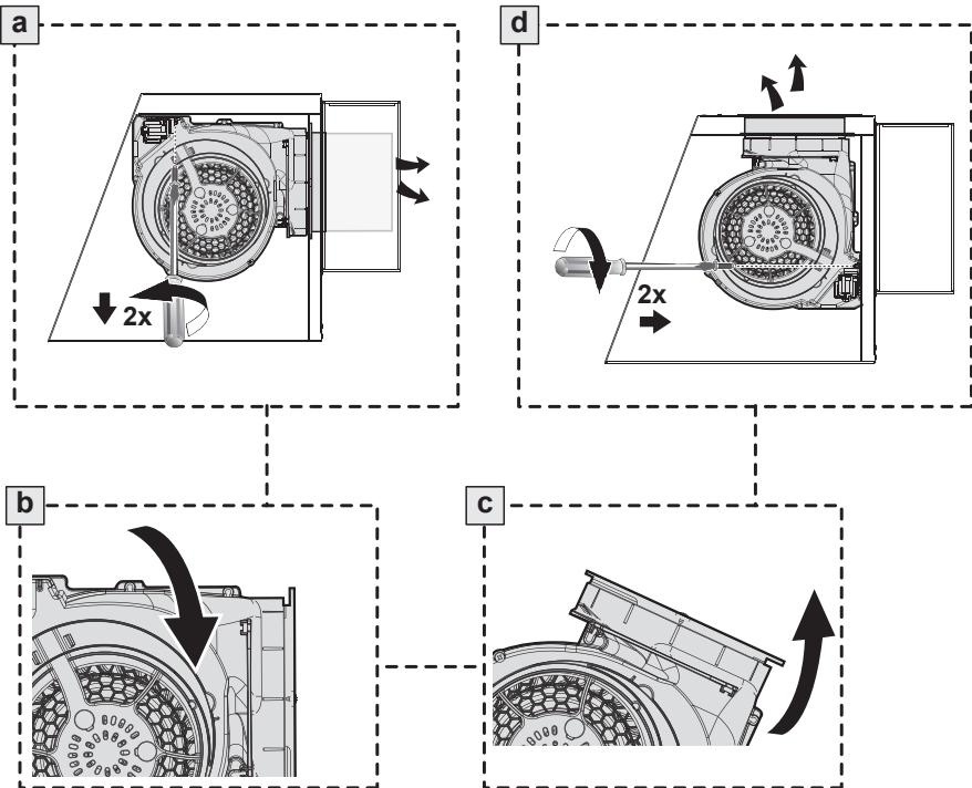
Unscrew the 2 screws that hold the blower and unlock it from the initial position as shown in Image a.
