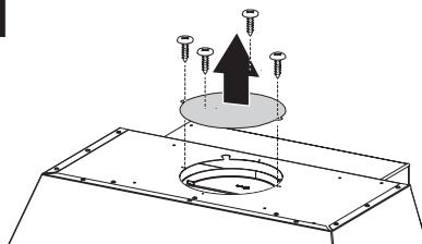
Remove the 4 screws as shown and take off the cover plates.
