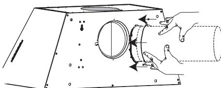
After fixing the Body Hood to the Rear Section, fix the Blower in the previously position with the same 2 screws.
