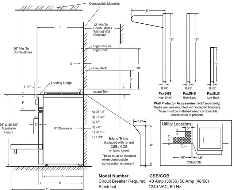
**GAS REQUIREMENTS :** 1/2" NPT gas connection. Minimum gas supply is 7" water column for natural gas and 11" for propane. Operating pressure at the manifold is 5" water column for natural gas and 10" for propane. All units include a gas regulator. The installer must provide a shut-off valve at the rear of the appliance with easy access to shut off the gas for service. High-altitude kits and gas conversion kits are available through the Capital parts department.
