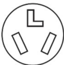
3-Wire receptacle (10-30R)
