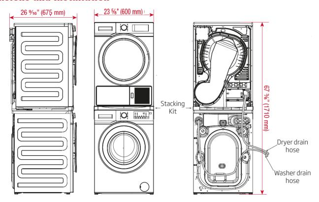
Stacked installation minimum air gap clearances: 6 ½" top, ½" sides, ½" back, front ½"
