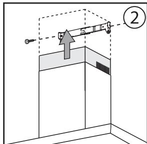
6. Insert top duct cover into bottom duct cover. Seat the duct covers correctly on the hood.
