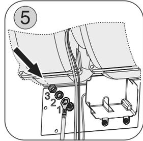
**WARNING!** Place electrical wiring inside the motor housing.
