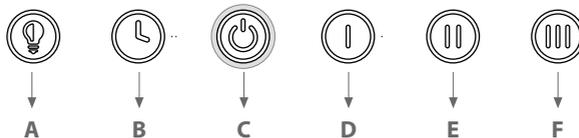
**A - Lights Button:** Lights are three level (high, medium, low). From stand-by-on mode, touch once for high, twice for medium, three times for low, four times to cycle back.
