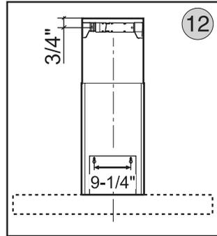
4. Secure duct cover bracket to top of wall just below the ceiling using (2) screws provided. See Fig.13
