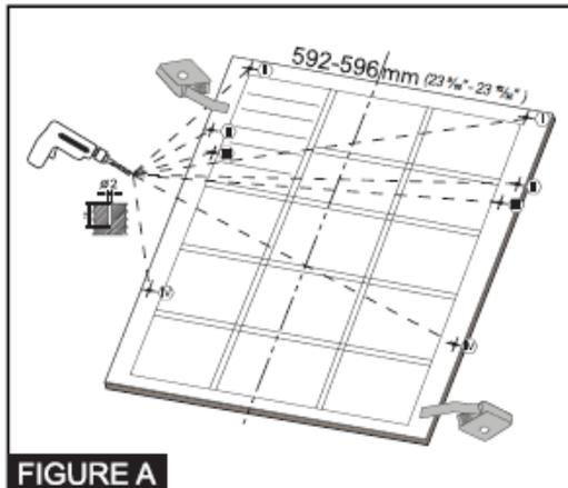
The mounting plan in the plastic bag is fixed to the inside of the Dishwasher door.
