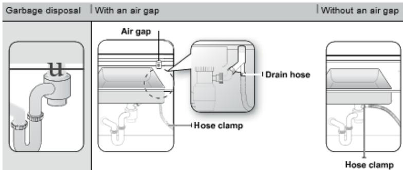
1. Check the size of the sink's drain hose connector. If needed, cut the drain hose so its end fits onto the sink connector (5/8 in., 3/4 in. or 1 in. - as shown in **C** below). If the end of the drain hose does not fit onto the drain hose connector of the sink, use an adaptor purchasable at a plumbing/hardware supply store.
