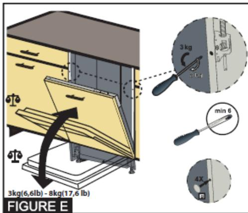
If the wooden door is falling down, the mechanism must be turned in the direction of the white arrow with a philips screwdriver.
