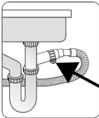
Use hose clamp that shown at the Figure 4. for drain hose assembly to the sink.
