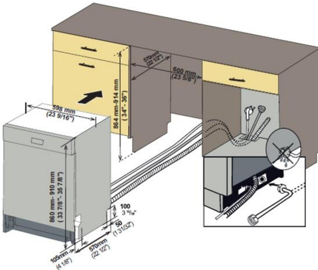
**CAUTION:** Make sure all hoses are pulled through the side opening of the cabinet. No hoses should be kinked and ensure all slack is taken out, as shown above.
