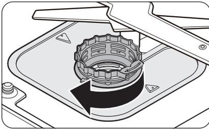
6. Reinsert the filter, and then the filter cover.
