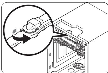
1. Check whether the nozzle holes are clogged by food particles.
