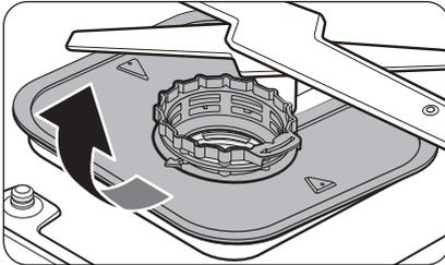
3. Remove the filter cover, and then the cylindrical micro filter underneath.
