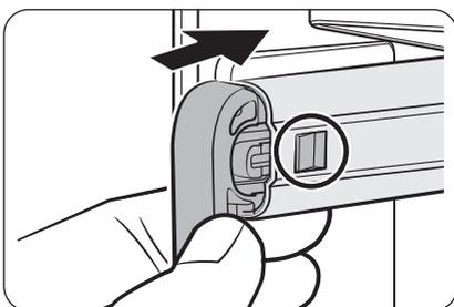
1. Stand facing the dishwasher, and then pull the 3<sup>rd</sup> rack out so that the handles at the ends of the rack supports (dark grey in the illustration) are even with the end of the rack.
