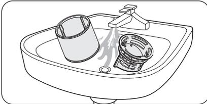
4. Remove any dirt and impurities from the micro filter and the filter cover.
