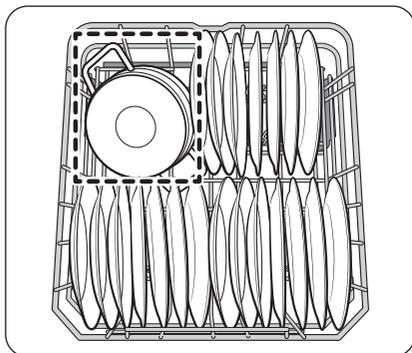
For more effective cleaning, load large items into the Storm Wash\* area on the left side of the lower rack (Dotted zone).
