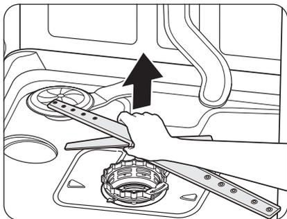
1. Open the door, and then pull out the lower rack to reveal the lower nozzle.
