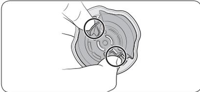
3. Remove the Coarse filter, and then the cylindrical micro filter underneath.
