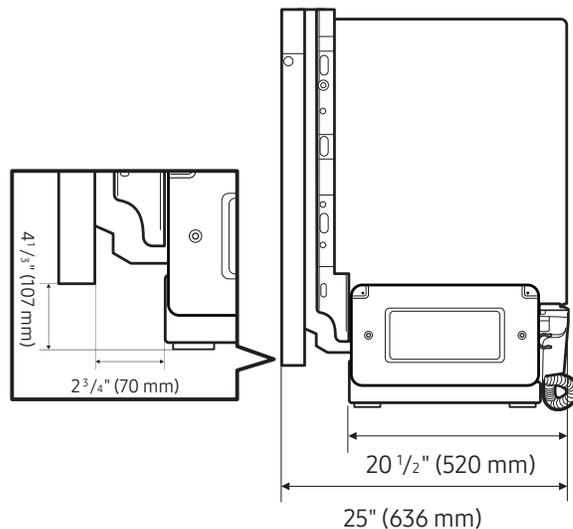
You must arrange the water supply line, power cable and drain hose in the space behind the dishwasher.
