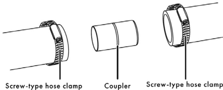
3. Secure the drain hose to the air gap, waste tee, or garbage disposal with a screw-type clamp, using the appropriate method below. See "Drain Preparation" on page 9 if you do not know which method to use.
