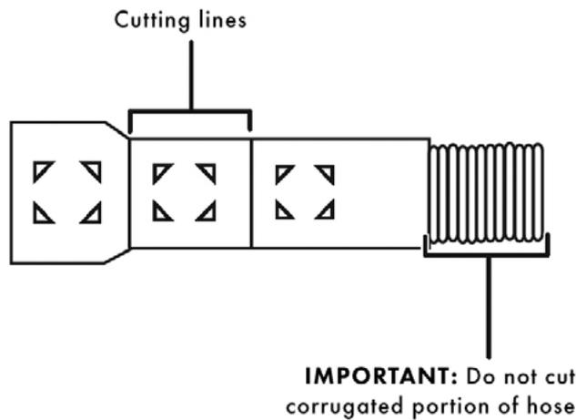
2. If a longer drain hose is required, you can add up to 42" (1067 mm) of length, for a total of 10' (3048 mm) to the factory installed hose. Use 5/8" (16 mm) or 7/8" (22 mm) inside diameter hose and a coupler to connect the two hose ends. Secure the connection with screw-type hose clamps.
