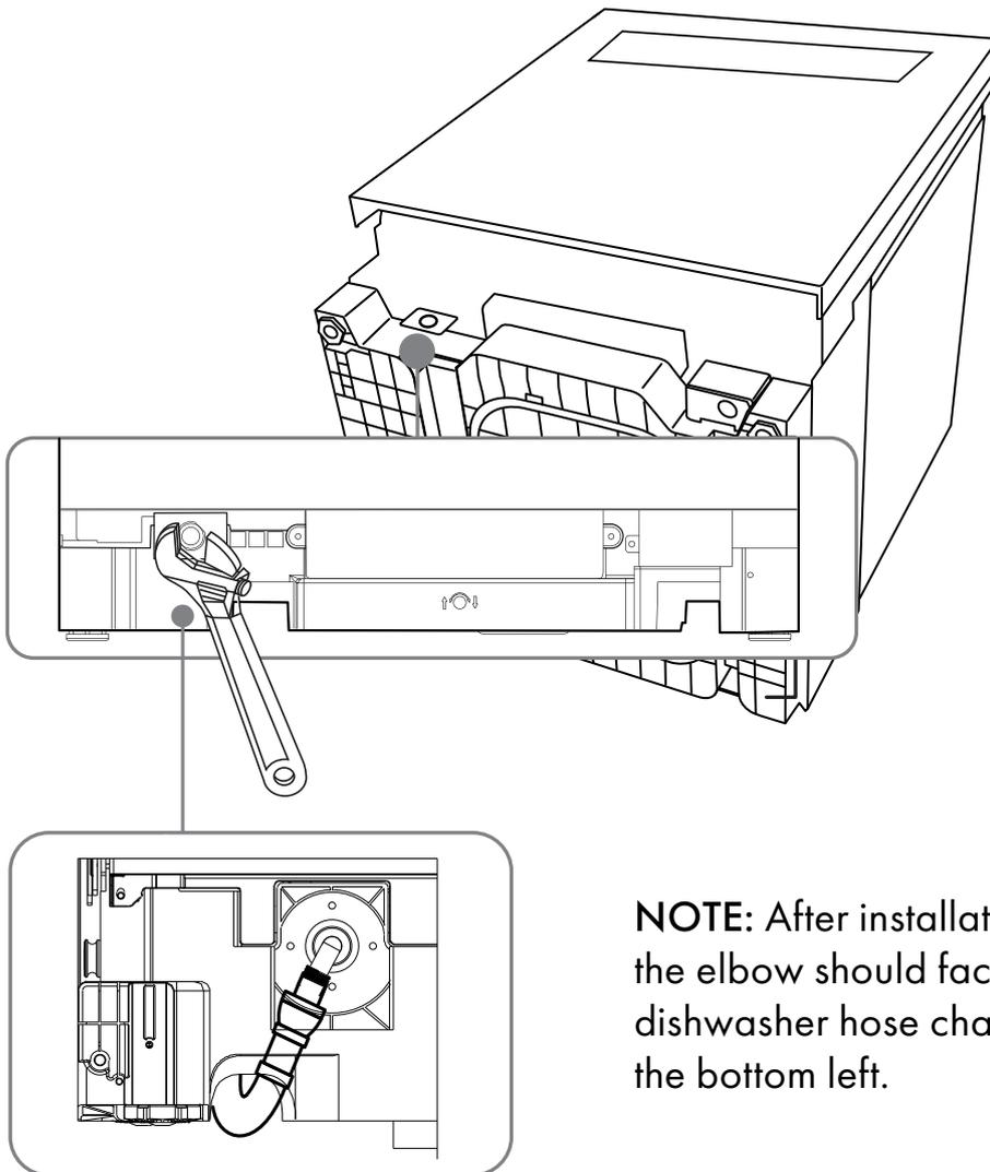
**NOTE:** After installation, the elbow should face the dishwasher hose channel at the bottom left.
