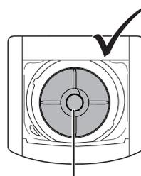
Washer is level - the water touches the leveling circle all the way around.
