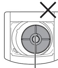
Washer not level - the water does not touch the leveling circle all the way around.
