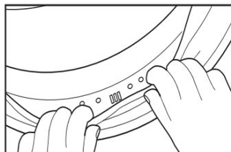
**NOTE:** Make sure nothing is blocking the holes behind the gasket.
