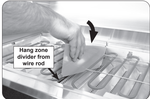
Fig. 34-3 Install zone divider
