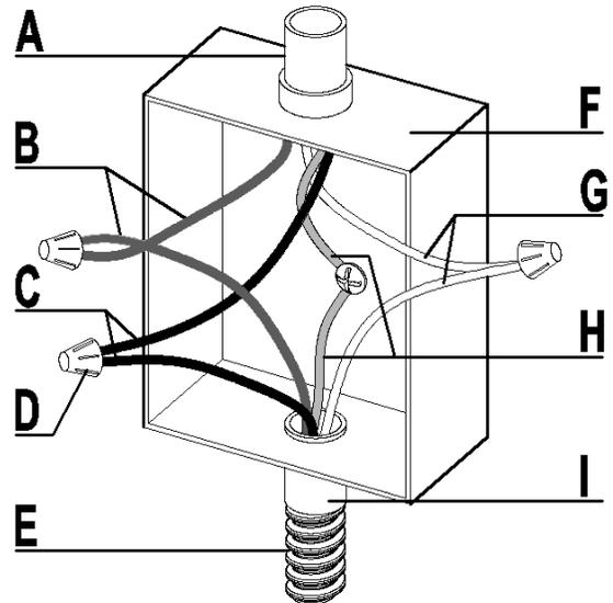
1. Connect the two black wires (C) together using a UL listed wire connector.
