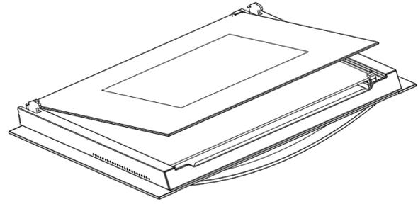
5. Lift the inside glass upwards as shown in the figure.
