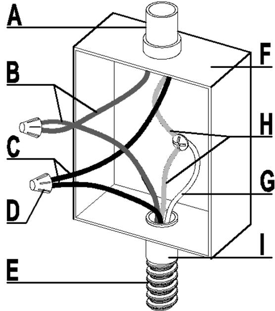
1. Connect the two black wires (C) together using a UL listed wire connector.
