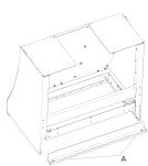
15. Only for ETRXXXXX hood models attach hood insert rear bracket support with 4 - 3.5 x 9.5 mm screws on the back.
