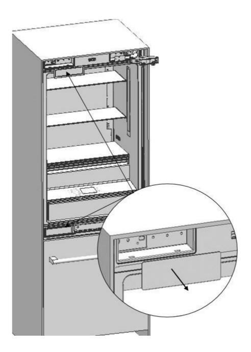
• Remove the lower right hinge by loosening its 2 screws and fix it to its slot at the upper left side.
