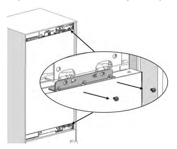
• Take out the fridge door and lay it down on a table remove the fixing parts and screw them to the opposite side of the door as shown figure.
