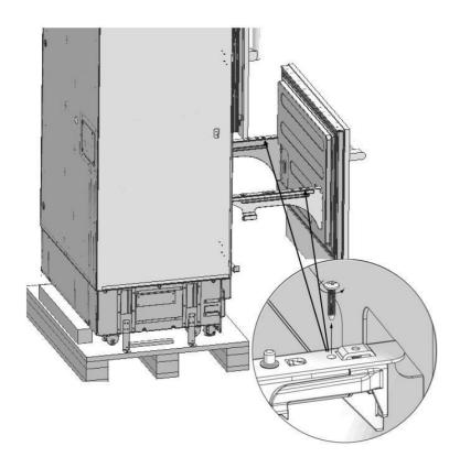
• Pull the door frontward to free it from the tabs at the back and remove it.
