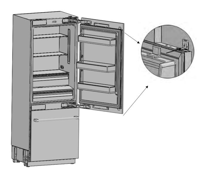
ER30SRB16IPR ER36SRB19IPR Attach and screw the upper/lower decoration cover.
