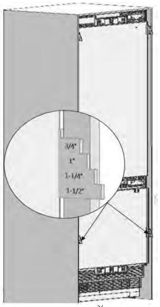
• The position adjustment jig (Item No5) must be adjusted according to the thickness of the door.
