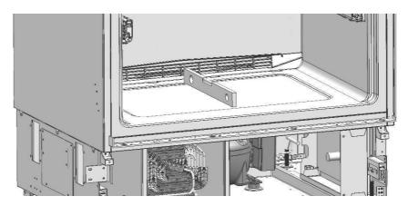
The maximum height that the adjustable feet can reach is 1 9/16" (40 mm) and the product height is 85 3/8" (2,169 mm)
