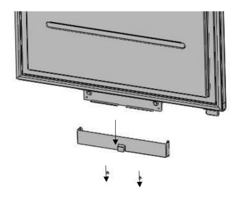
• Remove fridge lower and upper bracket and fixing screws.
