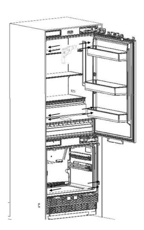
• Attach the cabinet- cabin connecting bracket to the furniture with 4screws.
