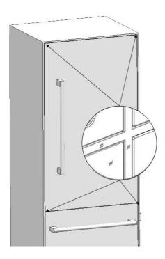
For products without furniture doors, the product is placed using the Adjustment part (Item No5) as shown in the figure below.
