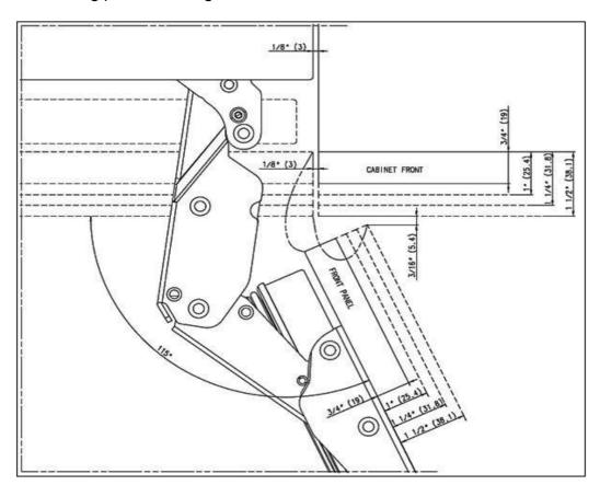
• You can limit the opening degree of your door to 90° if you want. In this case, the door thickness levels can be like the following (you can look at the relevant section to learn how to attach the 90° limiting pin (Item No6).
