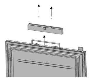
• Loosen 2 screws of the lower cover of the fridge door and remove it.
