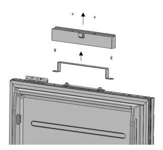
Remove two screws to take out the cover door hanger bracket low.
