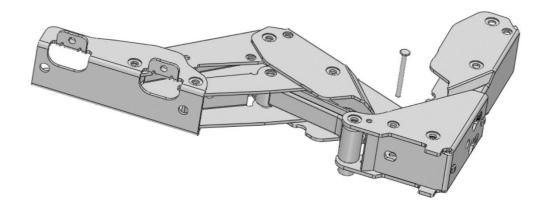
$90^{\circ}$  limit pin should be inserted to upper hinge and lower hinge
