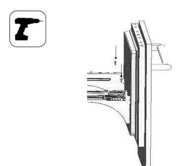
Locate the drawer onto the rail and tighten the screws
