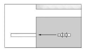
• Fit the anti tip brackets (item No.2) into their places, using 4 screws(item No.4) for each. You must use all of the 2 brackets to ensure safety of the product.
