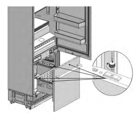
• Attach the cover freezing door top (Item No5) using the tabs.
