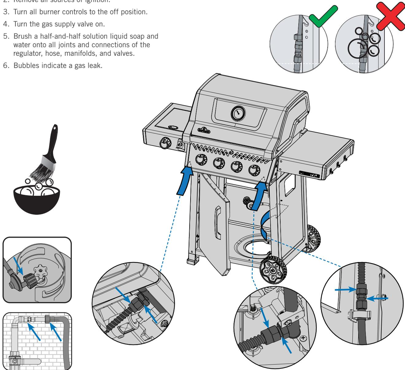
**WARNING!** Never use an open flame to check for gas leaks. Sparks or flames will cause a fire, explosion, damage to property, serious physical injury, or death.
