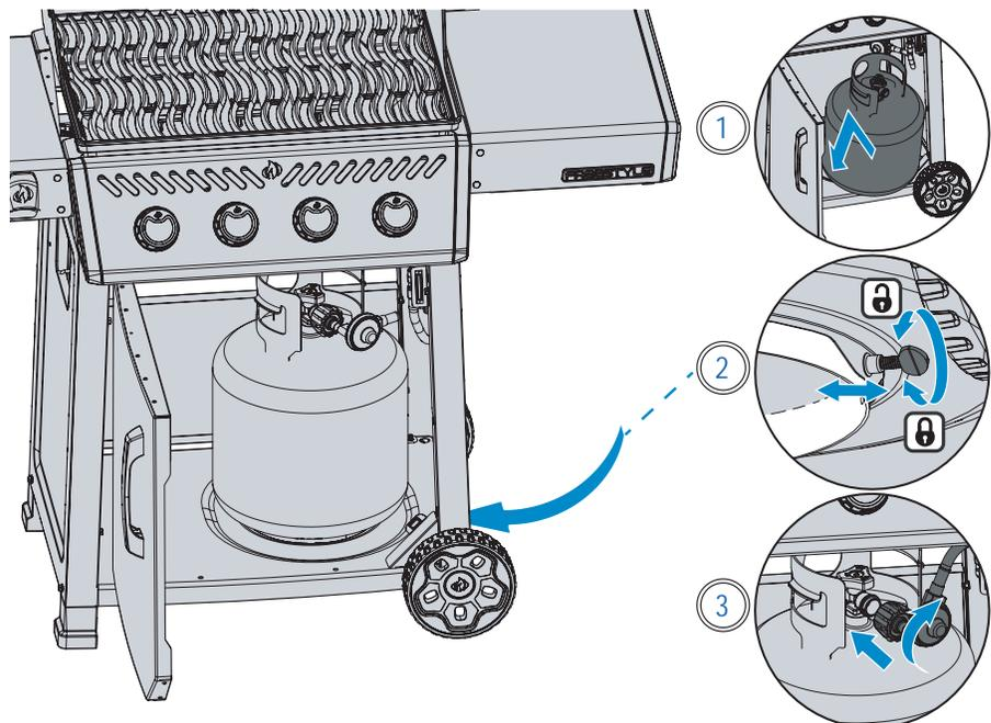
**WARNING!** Do not store a spare gas cylinder below the grill head or side burners.
