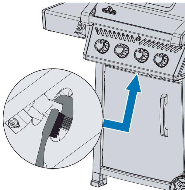
**WARNING!** It is very important the valve/orifice enters the burner tube when reinstalling the burner after cleaning and before lighting your grill, or a fire or explosion could occur.
