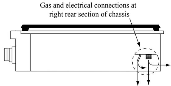
Gas connection and power cord may be routed through bottom or back of chassis
