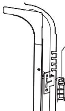
Open the door remove the tub cap on both sides of the tub. Install screw through the dishwasher side hole to the wall of cabinet. Reinstall tub cap.
