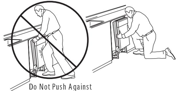
Do Not Push Against Front Door Panel With Knee. Damage to The Door Panel Will Occur.
