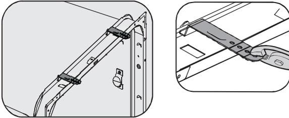
The dishwasher must be secured to the countertop. Position the dishwasher so that the tub flange aligns with the front face of the cabinet frame.
