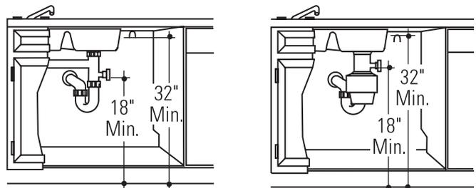
Install waste tee or disposer and air gap according to manufacturer's instructions.
