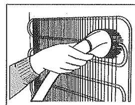
**CAUTION:** Failure to unplug the unit before cleaning or maintenance could result in electrical shock or personal injury.
