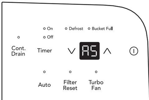
2. If the display reads "P2", Bucket is full or removed or not in right position. Replace the bucket in the right position.
