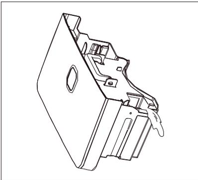
e. Replace the empty bucket back into the unit and once seated correctly, the unit will start up again.
