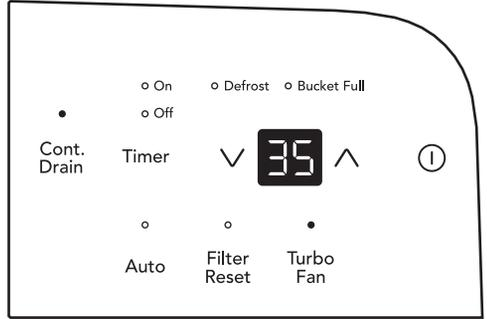
3. It is recommended to press the Cont. Drain button to use the CONTINUOUS setting for the first three or four days until the sweating and dampness odors have stopped. In this setting the unit will run in the maximum power and the display will show actual room humidity.
