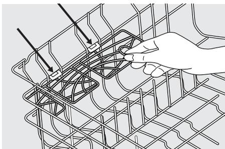
Place the clips of the cup shelf over the horizontal rack wires and push down to attach the cup shelf onto the second wire of the upper rack.
