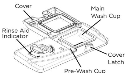
If the cover is closed on the Main Wash Cup open by pressing the Cover Latch.
