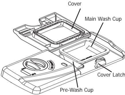
**If the cover is closed on the Main Wash Cup open by pressing the Cover Latch.**
