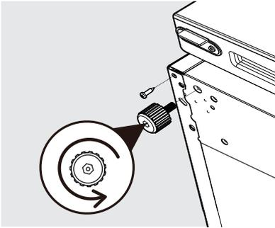
7. Attach the bottom hinge (A) with 4 screws (B) and the adjustable leveling foot (C) on the left side of the cabinet.
