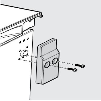
9. Using an adjustable wrench and pliers, move the hinge pin from the right side to the left side.
