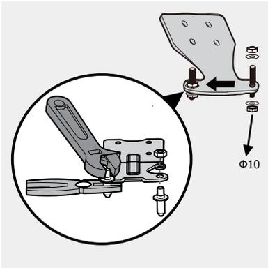
10. With a flat head screwdriver, gently pry upward on hinge pin bearing to remove from door. Reinstall on the opposite side of the door.
