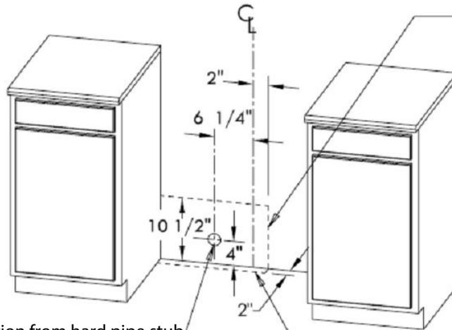
Area allows for flush installation with through-the-wall connection of pipe shut-off valve and rear wall 110/120V outlet.
