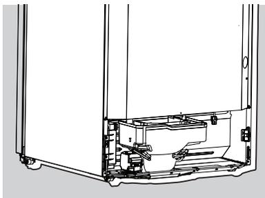
19. Remove the connector box from the unit with a Philips screwdriver. Discard screw. See Figure 15.
