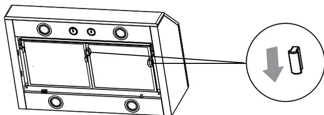
3. To clean grease filter, soak the filters in hot water using a mild detergent. Rinse well and shake to dry.
