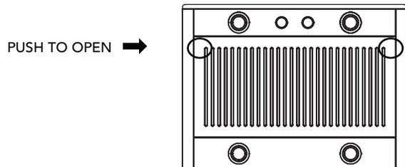
2. To remove or install the grease filters push tab towards the back of the unit.
