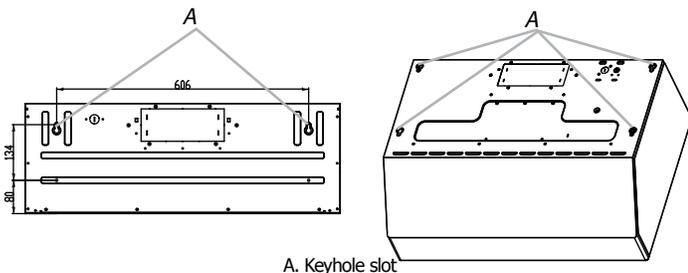
6. Use 5/64" drill bit and drill 4 pilot holes as shown for top range hood support.
