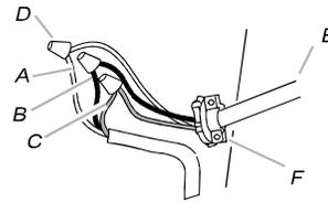
2. Use UL listed wire connectors and connect white wires (A) together.
