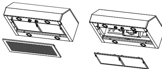
2. Remove the screws at the front support and slide the panel back.
