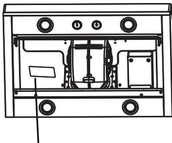
The serial plate is located on the left inside of the range hood
