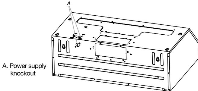
4. Lift the hood into final position. Feed enough electrical wire through the 1/2" UL listed or CSA approved strain relief to make connections in the terminal box. Tighten the strain relief screws.
