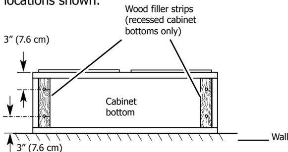
5. Lift the range hood up under cabinet and determine final location by centering beneath cabinet. Mark on the underside of cabinet the location of the 4 keyhole mounting slots on the range hood (See slot dimensions on page 6). Mark rear mounting screw hole locations. Set range hood aside on a covered surface.
