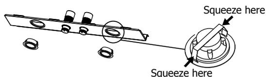
5. Replace with new LED lights Part number 5304503879 and re-install the front support
