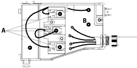
4. Connect the ground conductor (green wire) under the terminal B. Then connect the neutral wire (white wire) to center of the terminal. Neutral ground conductor of the dryer should remain on the center terminal. Be sure that neutral ground conductor of dryer and neutral wire of supply cord connected to center terminal together. Tighten all screws.
