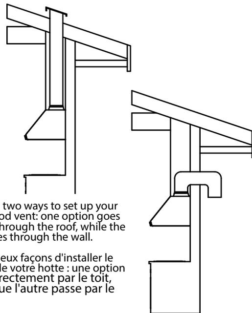
There are two ways to set up your range hood vent: one option goes straight through the roof, while the other goes through the wall.
