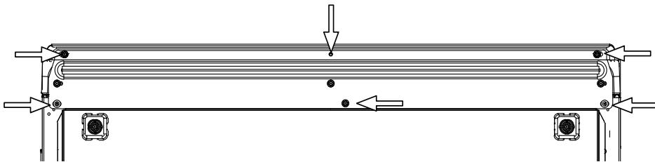
2. Align the holes in the backsplash with the holes in the oven.
