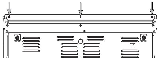
2. Line up the cutouts in the island trim piece onto the loosened screws and slide down into place.
