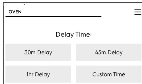
When the Delay Start time is reached, the oven will turn on and begin cooking. The screen will show the oven temperature.
