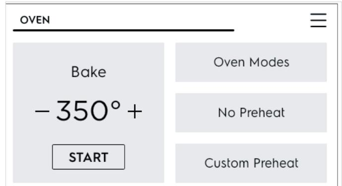
2. Touch **Oven Modes** and touch **Bake**. The default temperature 350°F will show in the display. You can also use the controls on the Quick Start screen.
