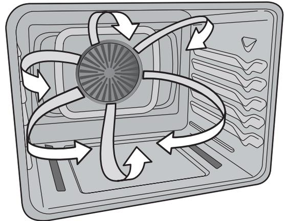
**Figure 6: Convection roasting on lower oven racks**
