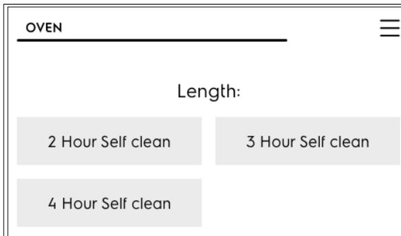
When the oven is set to run a self-clean cycle, the motor door lock will begin locking the oven door. Do not open the oven door while the lock motor is running or when any locking indicators or displays are showing. The oven door is completely locked in about 4 seconds. Once the oven door has locked, CLEAN will appear in the display indicating self clean has started.
