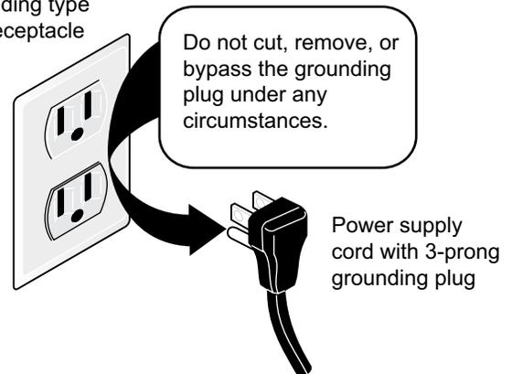
This appliance is equipped with a 3-prong grounding plug for your protection against shock hazard and should be plugged directly into a properly grounded receptacle. Do not cut or remove the grounding prong from this plug.
