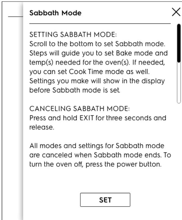
To exit Sabbath Mode, press and hold **EXIT** for three seconds.
