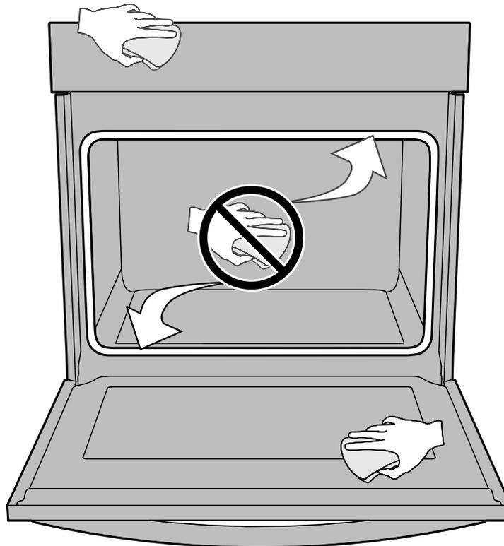
**Figure 11: Do not clean oven door gasket**
