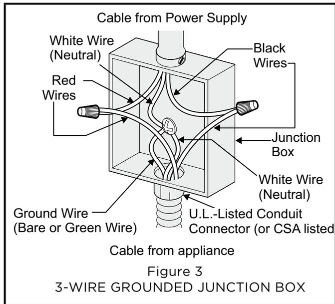
If oven is used in a new branch circuit installation (1996 NEC), mobile home, recreational vehicle, or where local codes DO NOT permit grounding through the neutral (white) wire, the appliance frame **MUST NOT** be connected to the neutral wire of the 4-wire electrical system (see Figure 4):
